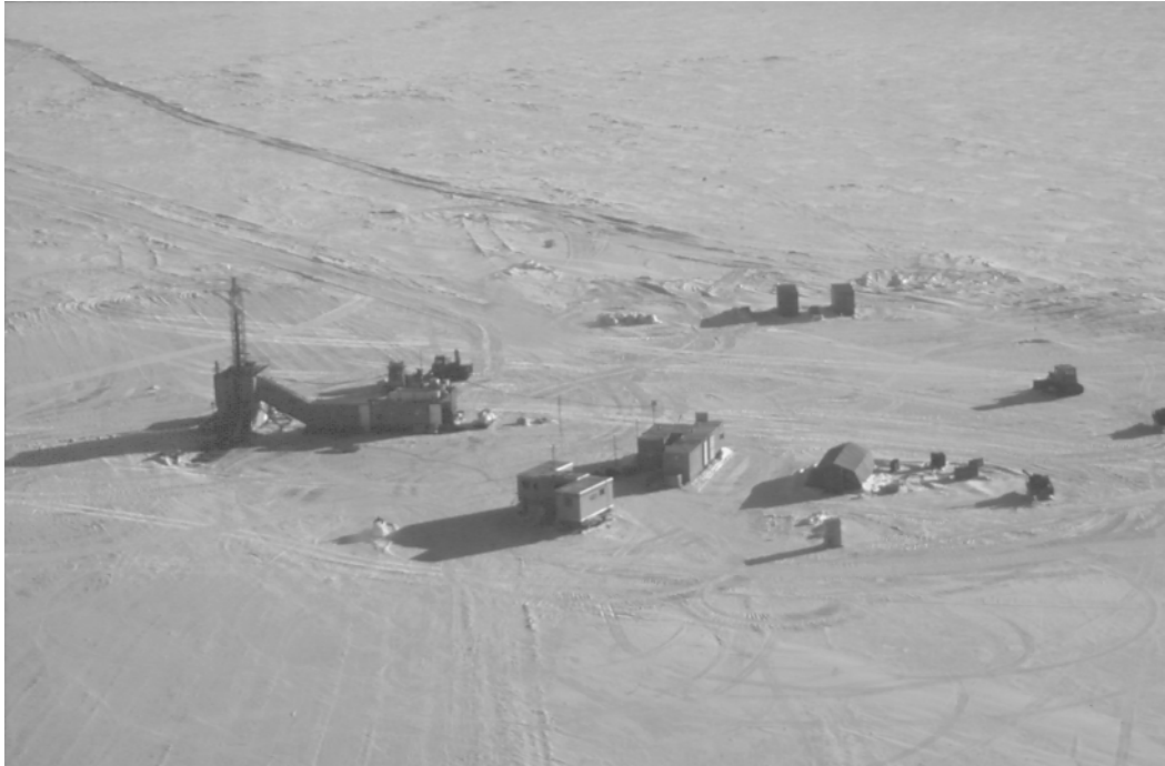
Fig. 1.11 - Aerial of view the CRP-3 drill site to show the layout of the rig, with sloping covered ramp down to the mudroom, and with core processing and physical properties laboratories in a cluster 30 m to the right. Photo: P.J. Barrett.
