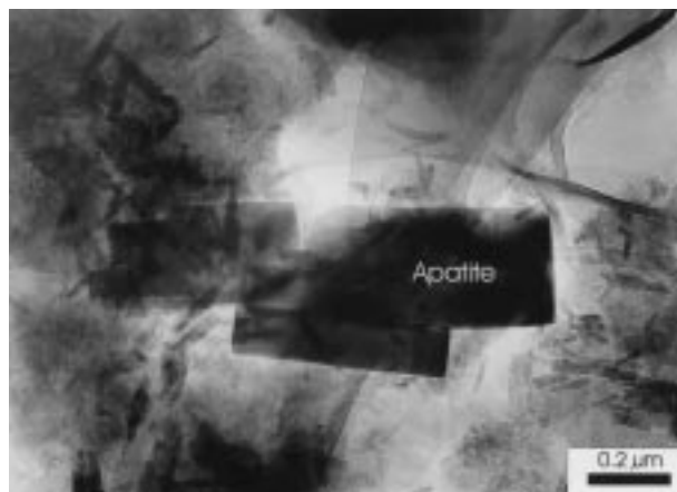
Fig. 10 - Core level 901.2 mbsf, TEM image showing an assemblage with apatite, smectite, feldspars, kaolinite and halite.
